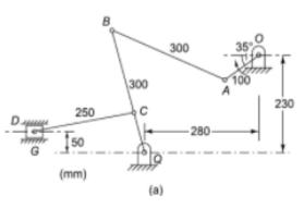
(c) State kennedy theorem. Locate all instantaneous centre of rotation for a four-bar mechanism.
