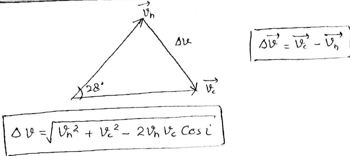
If the line connecting to opposite perigee is the node line and the inclination correction is made at the apogee in connection with orbit circularization, Then-
