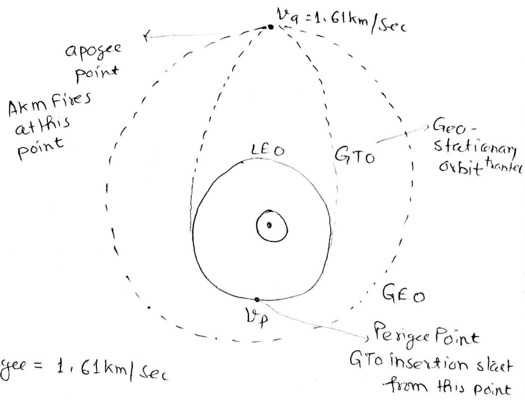
$$V_a = \text{Velocity at apogee} = 1.61 \text{ km/sec}$$
