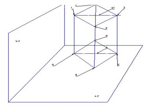
EX.1 A square base pyramid side 40 mm and height 85 mm axis perpendicular HP and parallel to VP. Draw the projection. (all base side are equally inclined to the VP)
