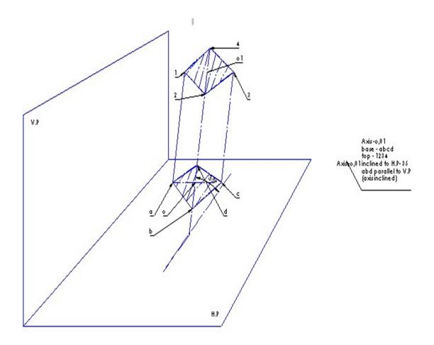
Ex.1 A square base pyramid side 40 mm and height 85 mm axis inclined to HP 38<sup>°</sup> and parallel to VP. Draw the projection. (all base side are equally inclined to the VP)
