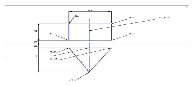
Ex.2 A Hexagonal base pyramid side 40 mm and height 65 mm axis parallel to HP. Draw the projection
