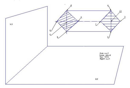
Ex.1 A square base pyramid side 40 mm and height 65 mm axis parallel to HP. Draw the projection.
