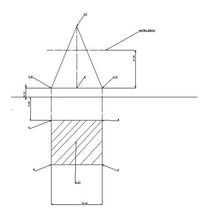
Case 2 – axis perpendicular to HP and cut by a section Plane and section plane parallel to VP.
