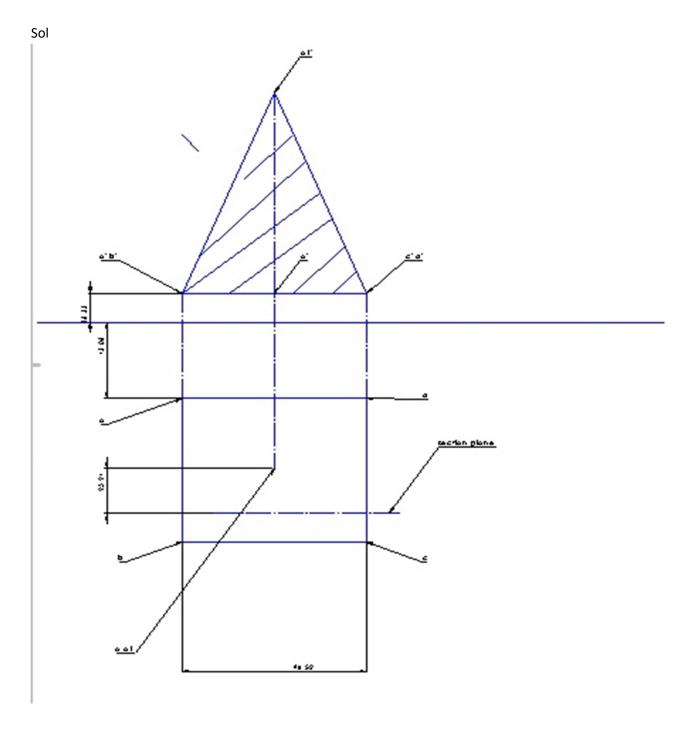
Case 3 – axis perpendicular to HP and cut by a section Plane and section plane inclined to HP.
