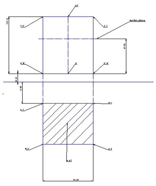
Q.2 **Q.1** A square base pyramided side 96 mm and height 119 mm ,axis perpendicular to HP cut by a section plane, section plane parallel to HP and cut the axis 45 mm above the base.
