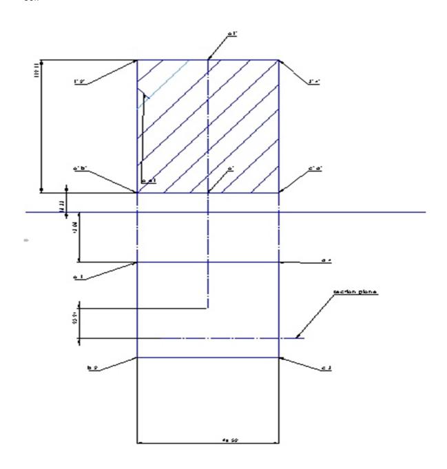
Q.2 A square base pyramided side 96 mm and height 119 mm ,axis perpendicular to HP cut by a section plane, section plane parallel to VP and cut the axis 25 mm away the center.
