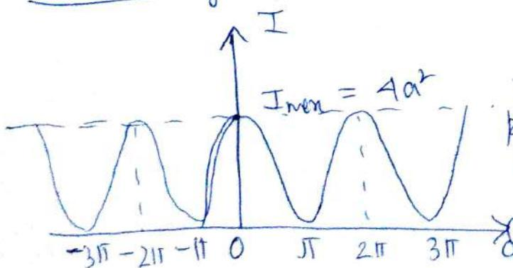
A curve showing the variation of intensity with phase is called intensity distribution curve.
