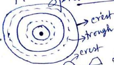
Waves from a pt. source in a uniform isotropic medium is shown in the figure. In isotropic medium the light waves travel in all directions and hence the locus of all points which have the same amplitude and are in same phase is a sphere. Thus each spherical surface concentric with the source is a wave front. At large distances from the source, a small portion of the spherical wave front can be considered as plane wave front.
