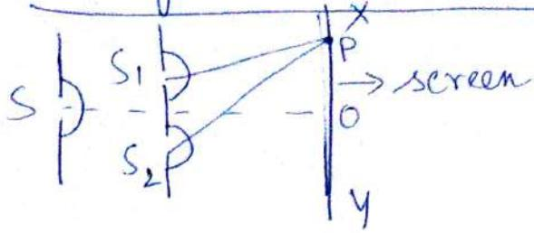
Let  $S$  be the source of monochromatic light of wavelength  $\lambda$ .  $S_1$  and  $S_2$  are two pinholes or slits which are situated at equidistant from the source. The waves arriving at  $S_1$  and  $S_2$  from  $S$  will be in phase at all time and having same frequency. The secondary waves coming out from  $S_1$  and  $S_2$  superimpose with each other and interference pattern is formed on the screen. We have to investigate the intensity at  $P$  on the screen  $XY$ .
