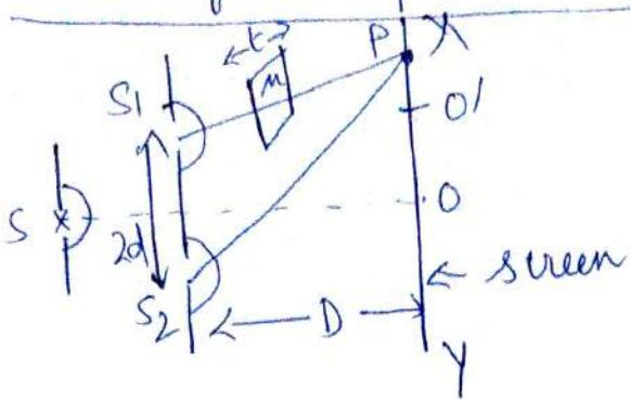
Let us now discuss the change in the interference pattern produced by introducing a thin transparent plate in the path of one of the two interfering beams as shown in the figure.
