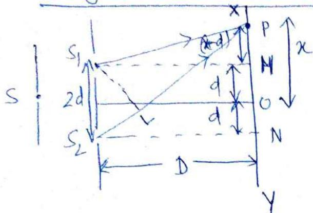
Let  $S$  be a narrow slit which is illuminated by the monochromatic light of wavelength  $\lambda$ . The two slits  $S_1$  and  $S_2$  are separated by a distance  $2d$ . Let a screen  $XY$  be placed at a distance  $D$  from the coherent sources  $S_1$  and  $S_2$ . Waves coming out from  $S_1$  and  $S_2$  are intercepted on the screen  $XY$ . Now we will find out the positions of maxima (bright fringe) and minima (dark fringe) on the screen.
