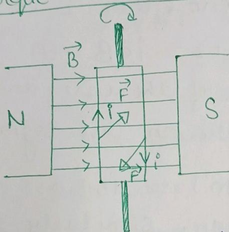
An electric motor. Loop carries an electric current. the magnetic forces on the long sides of the loop produces a torque that tends to rotate the loop clockwise.
