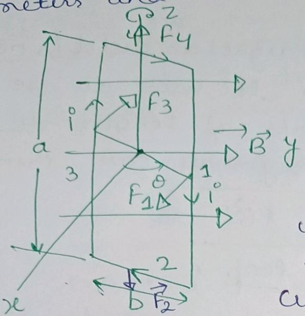
We consider a rectangular loop of length  $a$  and width  $b$  carrying a current  $i$ . The plane of the loop makes an angle  $\theta$  with the  $x$ -axis.
