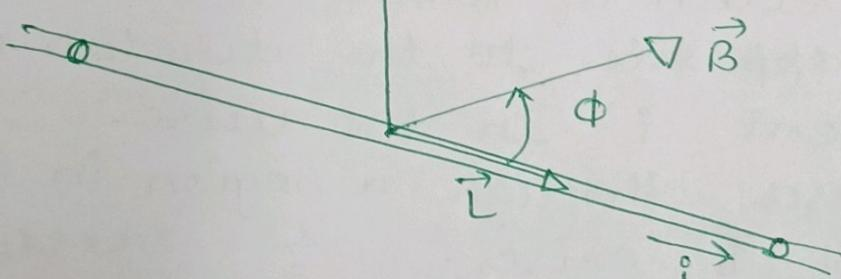
If the field is uniform over the length of the wire segment and the direction of the current makes an angle  $\phi$  with the field, then the magnitude of the force is
