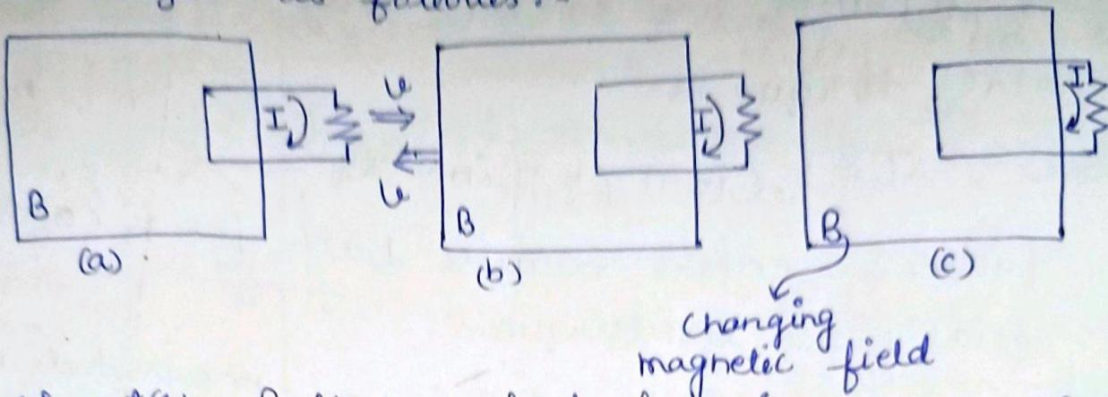
Experiment(1) Pulled a loop of wire to the right through a magnetic field (a). A current flowed in the loop.
