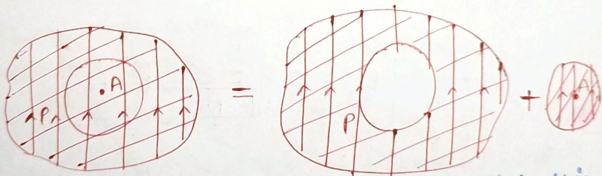
the field at any point  $A$  in a dielectric can be considered as the sum of the field in a spherical hole plus the field due to a spherical plug.
