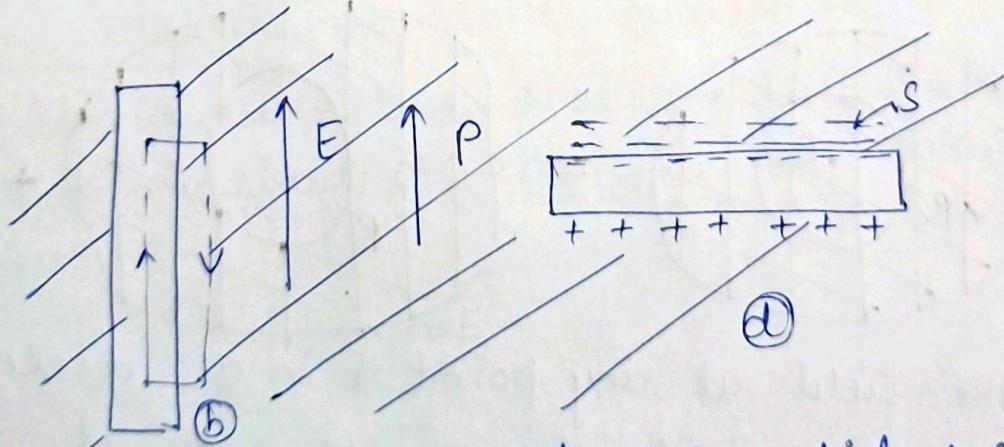
The field in a slot cut in a dielectric depends on the shape and orientation of the slot.
