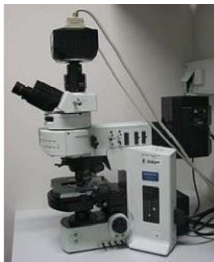
Figure 3 An upright fluorescence microscope (Olympus BX61) with the fluorescent filter cube turret above the objective lenses, coupled with a digital camera.
