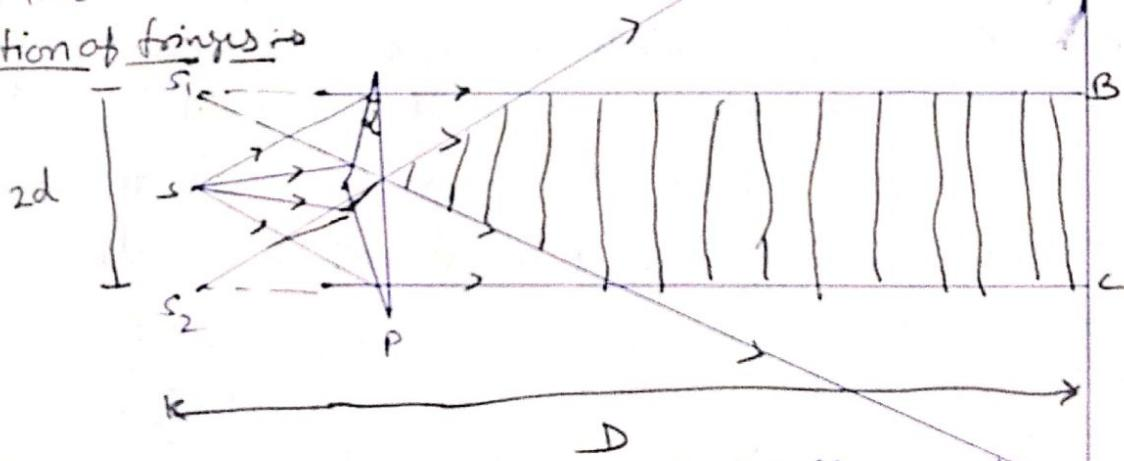
In above fringe S is a narrow vertical slit illuminated by monochromatic light the light from S is allowed to fall symmetrically on the biprism P placed at a small distance from S and having its refracting edge parallel to the slit. The light beams emerging from the upper and lower part of the prism appear to start from two virtual image of S namely  $S_1$  and  $S_2$ , which act as coherent sources.
