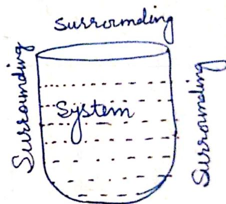
Types of systems: Sys may be classified into three types depending on the movement of matter and energy in or out of the system.
