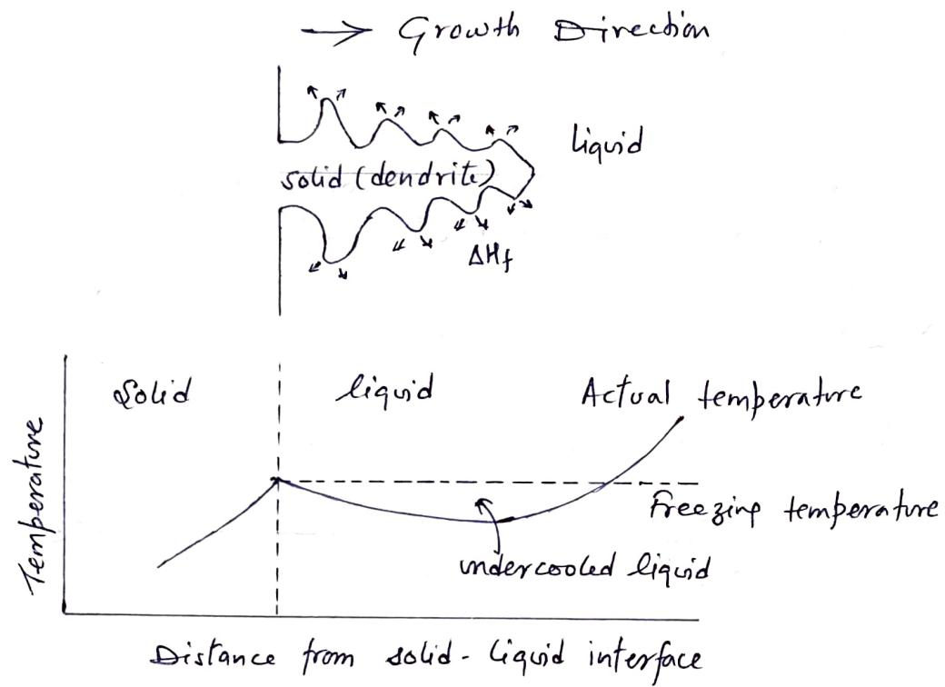
Fig 6 : If the liquid is undercooled, a protuberance on the solid- liquid interface can rapidly grow as a dendrite. The Latent heat of fusion is removed by raising the temperature of the liquid back to the freezing temperature.
