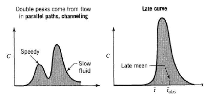
Late tracer is puzzling. Material balance says it can't happen so the only explanations are:  $\mathbf{v} \text{ or } \mathbf{V}$  are incorrectly measured (check flow meters) tracer is not inert (adsorbs on surface? Try a different one) the closed vessel assumption is far from satisfied.
