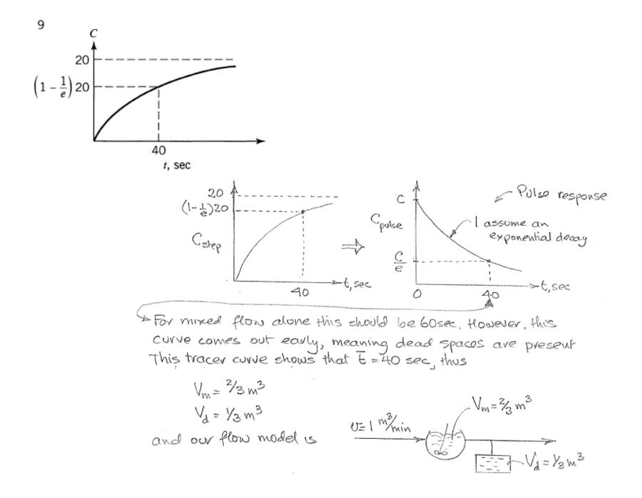
12.11. The second order aqueous reaction  $A + B \rightarrow R + S$  is run in a large tank reactor ( $V = 6 \text{ m}^3$ ) and for an equimolar feed stream ( $C_{A0} = C_{B0}$ ) conversion of reactants is 60%. Unfortunately, agitation in our reactor is rather inadequate and tracer tests of the flow within the reactor give the flow model sketched in Fig. P12.11. What size of mixed flow reactor will equal the performance of our present unit?
