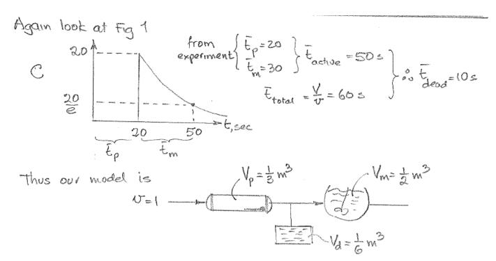
12.7. to 12.10. A step input tracer test (switching from tap water to salt water, measuring the conductivity of fluid leaving the vessel) is used to explore the flow pattern of fluid through the vessel ( $V = 1 \text{ m}^3$ ,  $v = 1 \text{ m}^3/\text{min}$ ). Devise a flow model to represent the vessel from the data of Figs. P12.7 to P12.10.
