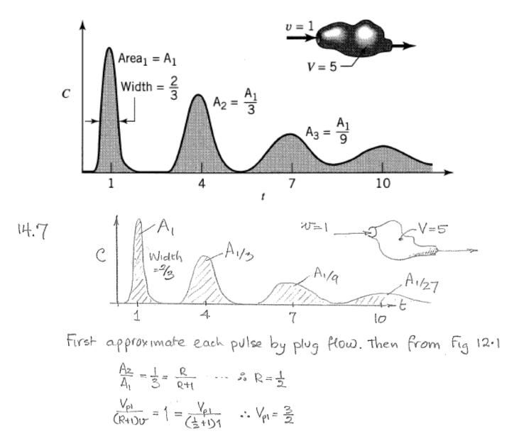
$$\frac{V_{p1}}{(R+1)V} + \frac{V_{p2}}{RV} = 3 = \frac{3/2}{(V_2+1)1} + \frac{V_{p2}}{(V_2)1}$$
