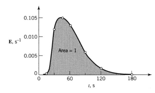
$\Delta \overline{t} = 280 - 220 = 60 \text{ s}$  $\Delta (\sigma^2) = 1000 - 100 = 900 \text{ s}$
