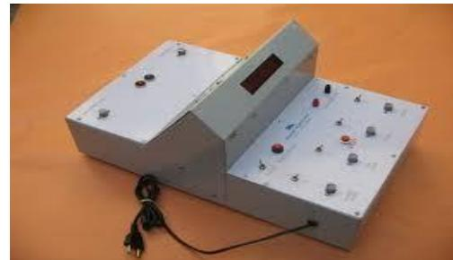
The simplest method of reducing reaction time is to have a subject place his finger on a button pressing with instructions to remove his finger when he sees a light signal just above the button. The apparatus used is called as chronoscope.
