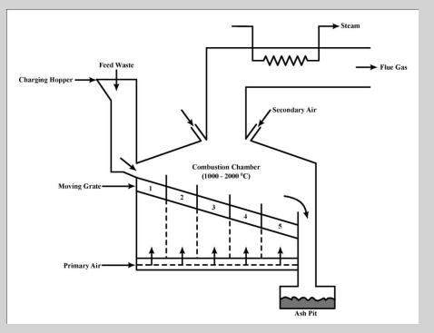
• A single moving grate boiler can handle up to 35 metric tons/hr of waste and can operate 8,000 hr/year with single stop for inspection and maintenance of about one month duration.
