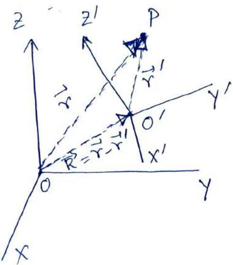
Two observers  $O$  and  $O'$ , fixed relative to two coordinate systems  $Oxyz$  and  $O'x'y'z'$  respectively, observe the motion of a particle  $P$  in space. We have to show that to both the observers the particle  $P$  appears to have the same force acting on it if and only if the two coordinate systems are moving at constant velocity relative to each other.
