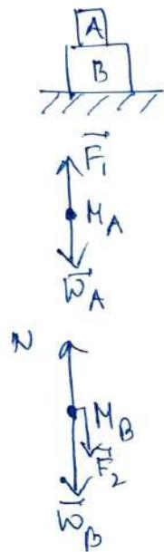
For example, in the case of two blocks on the table,  $\vec{F}_1$  is the force exerted by block B on block A and  $\vec{F}_2$  is the force exerted by block A on block B. Hence for Newton's 3rd law of motion  $\vec{F}_1 = -\vec{F}_2$  i.e.,  $|\vec{F}_1| = |\vec{F}_2|$ .
