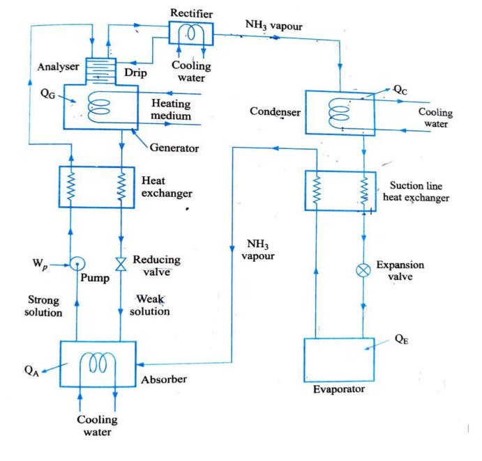
**1. Heat exchanger**. A heat exchanger is located between the generator and the absorber. The strong solution which is pumped from the absorber to the generator must be heated ; and the weak solution from the generator to the absorber must be cooled. This is accomplished by a heat exchanger and consequently cost of heating the generator and cost of cooling the absorber are reduced.
