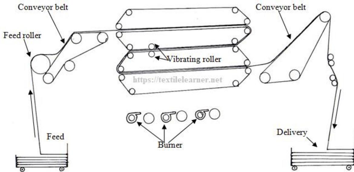
Fig: Schematic diagram of dryer with fabric path
