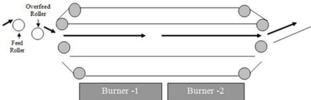
Fig: Passage Diagram of The fabric in Dryer Machine.
