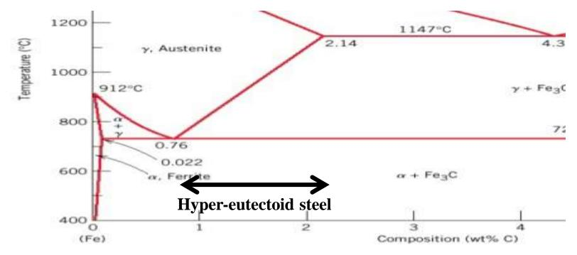
➢ If a Hyper-eutectoid plain carbon steel is heated to austenitic temperature for a sufficient time, it's structure will become Homogeneous austenite. This Process is called Austenitizing.
