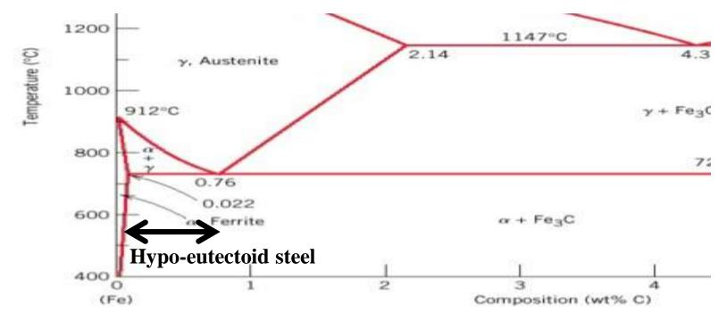
➢ If a Hypo-eutectoid plain carbon steel is heated to austenitic temperature for a sufficient time, it's structure will become Homogeneous austenite. This Process is called Austenitizing.
