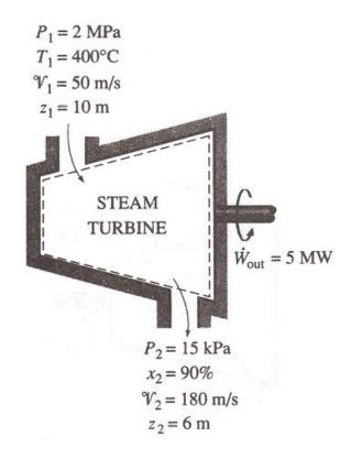
We take the turbine as a system. The control volume is shown in the figure. The system, the inlet and exit velocities do work and elevations are given and thus the kinetic and potential energies are to be considered.
