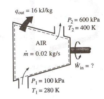
We take the compressor as the system. This is a control volume since the mass crosses the system boundary during the process. Heat is lost from the system and work is supplied to the system.
