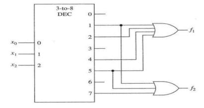
Implementation of a Full Adder circuit using Decoder.
