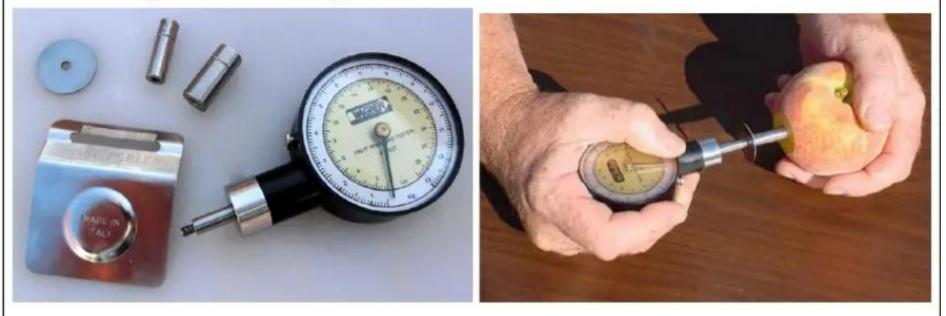
•Plunger of variable diameter is pressed into the fruit to a given depth.
