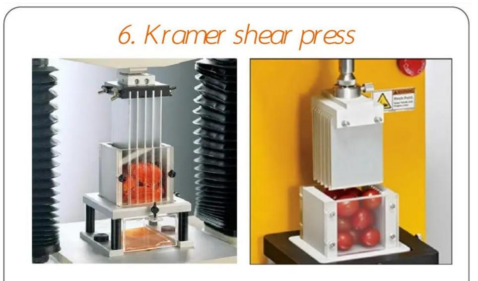
Many test cell assemblies with same power supply, to test the tenderness
