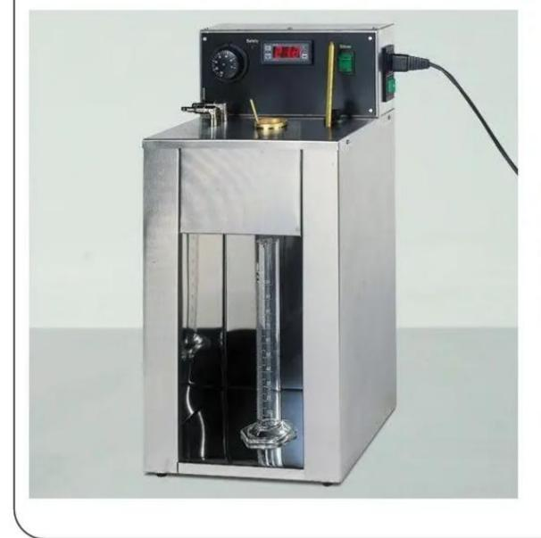
Measures the time necessary for a quantity of fluid to pass through an orifice or capillary under standard pressure
