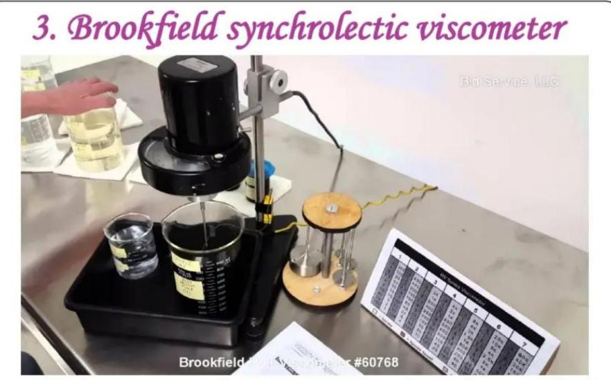
Based on the measurement of resistance to rotation of a spindle immersed in the test material
