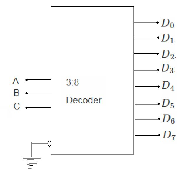
It is also called a binary-to-octal decoder since the inputs represent 3bit binary numbers and the outputs represent the eight digits in the octal number system.
