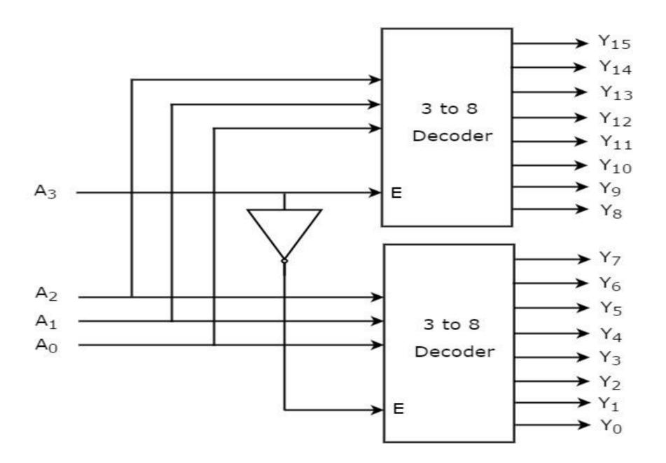
The parallel inputs  $A_2$ ,  $A_1 & A_0$  are applied to each 3 to 8 decoder. The complement of input, A3 is connected to Enable, E of lower 3 to 8 decoder in order to get the outputs,  $Y_7$  to  $Y_0$ . These are the **lower eight min terms**. The input,  $A_3$  is directly connected to Enable, E of upper 3 to 8 decoder in order to get the outputs,  $Y_{15}$  to  $Y_8$ . These are the **higher eight min terms**.
