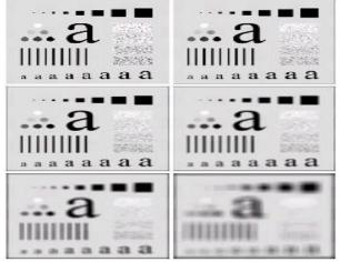
A major application of smoothing is noise reduction but because edge are also provided using sharp transitions so smoothing filters have the undesirable side effect that they blur edges. It also removes an effect named as false contouring which is caused by using insufficient number of gray levels in the image.
