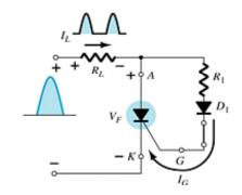
In this example, the SCR fires later—at the 90° point—on the positive half-cycle.
