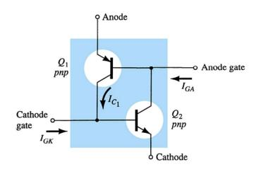
Note: The anode gate requires higher voltages than the cathode gate.
