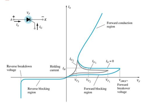
An SCR cannot be switched off by simply removing the gate voltage.
