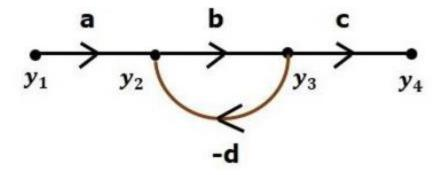
The nodes present in this signal flow graph are y1, y2, y3 and y4.
