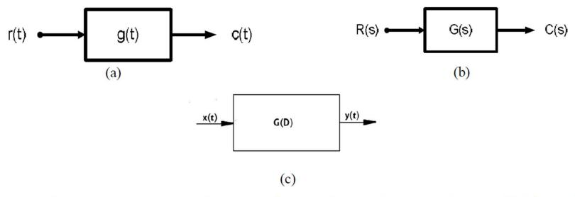
(a) A system in time domain, (b) a system in frequency domainand (c) transfer function with differential operator
