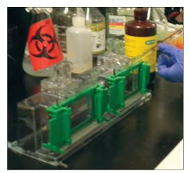
Figure 2: Add gel solution using a transfer pipette
