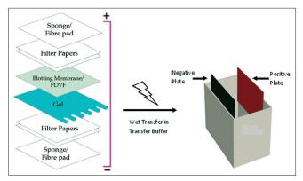
Figure 12: Assembly of a sandwich in western Blot
