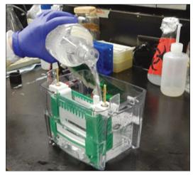
Figure 3: Add running buffer to the electrophorator
