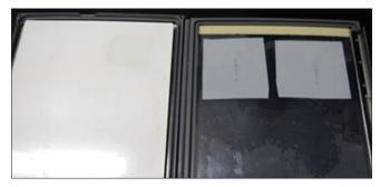
Figure 11: Use the cassette to expose the membrane in the dark room
