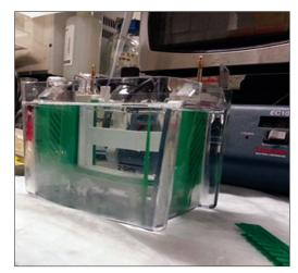
Figure 4: Add samples and molecular marker to the gel, after removing the combs
