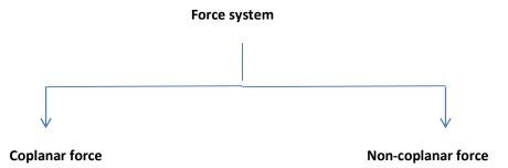
(When all the force lies in a single plane then That (when all the force lies in different plane that force force system is called coplanar) system is called non- coplanar force system)
