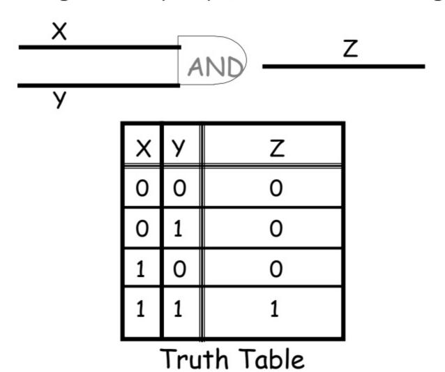
AND Gate is a circuit that allows output current to flow if both inputs are flowing.
