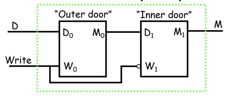
Two-Stage System to prevent feedback loop.
