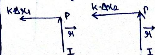
$$-k(r_1+a) [\Delta x_1 + \Delta x_2] = I\ddot{\theta} \quad \text{--- } ①$$
