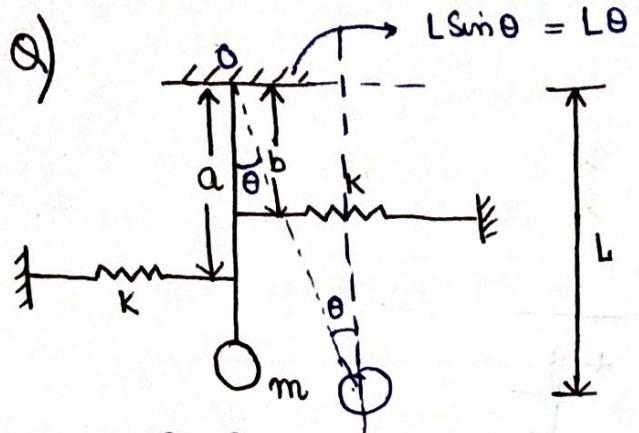
Displace pendulum by  $\theta$   $[\theta \approx \text{small}]$
