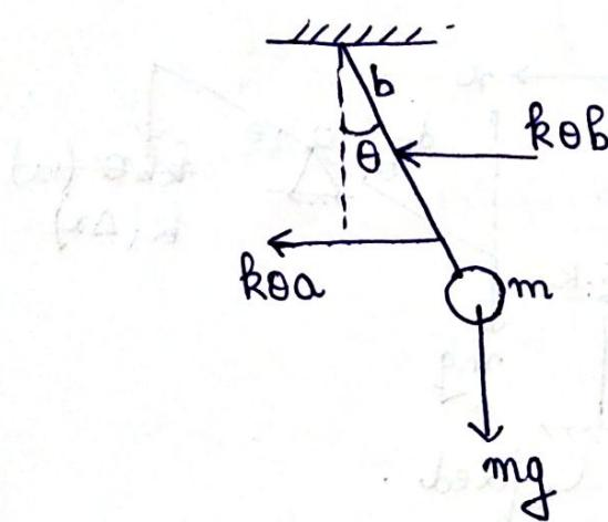
$$\text{Force} = \text{stiffness} \times \text{displacement}$$
