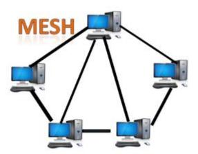
Mesh technology is an arrangement of the network in which computers are interconnected with each other through various redundant connections.
