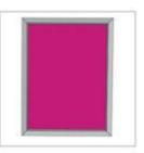
Step Three Mesh screen is coated with light sensitive emulsion.
